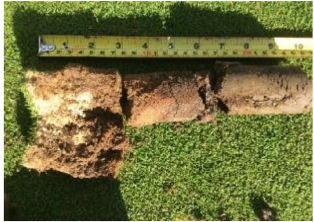
Figure 2: A clean and full fill of sand integration into the hollow core holes has been achieved. The 18<sup>th</sup> green, soil based profile, clearly shows the heavy texture soils, present from 170mm depth, which offer limited drainage potential.
